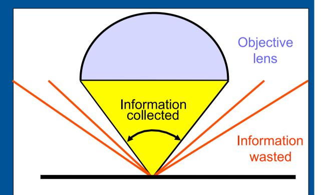
Illuminate the objective aperture uniformly over a controllable angle?
