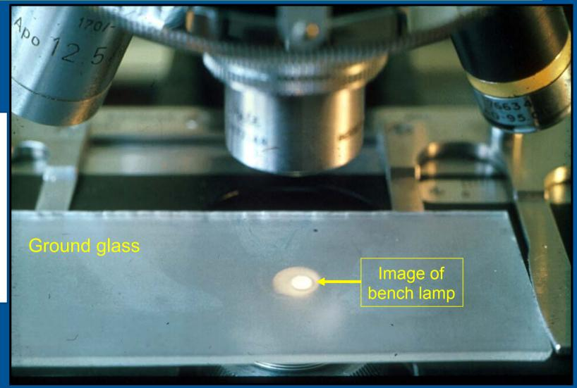
Bench lamp imaged on ground glass on stage by condenser lens
