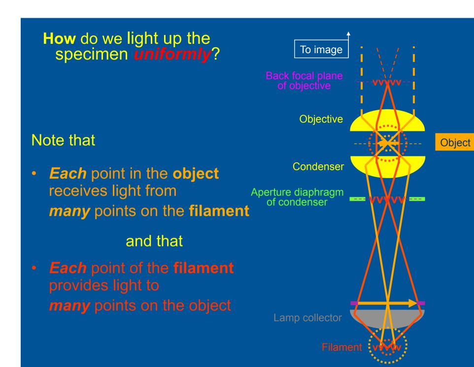
Illuminate the objective aperture uniformly over a controllable angle?
