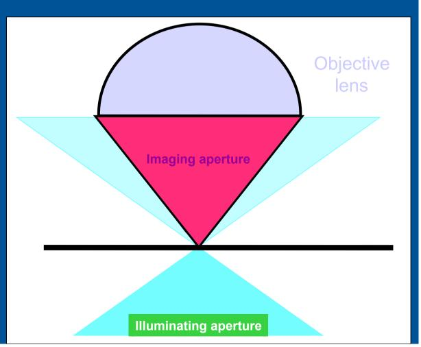
Illuminate the objective aperture uniformly over a controllable angle?
