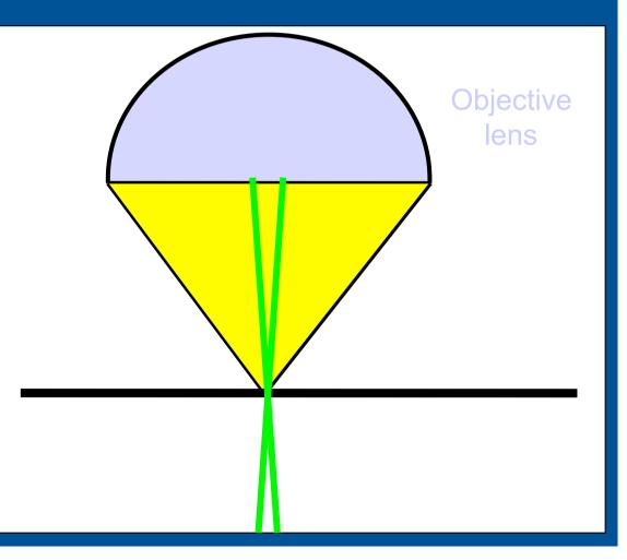
Illuminate the objective aperture uniformly over a controllable angle?
