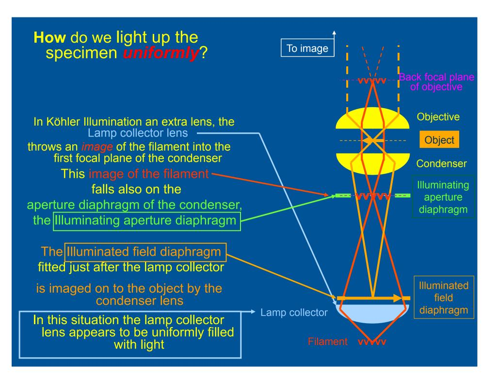
Light up the specimen uniformly over an *adjustable area*?
