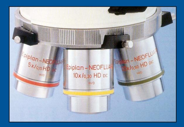
Magnification10xNumerical Aperture0.30'Hell- und Dunkelfeld'Suitable for Differential Interference ContrastCorrected for infinite tubelengthCorrected for use without coverglass
