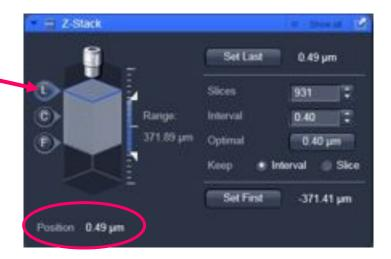
7. For the next sample, focus to the surface of the sample and set the position to "0". Stay at this position when reusing the image parameters of the stored image.
