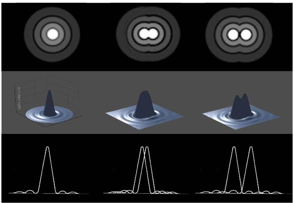
RESOLUTION is not a measure of how small an object we can see, it is the ability to distinguish which are closer together
