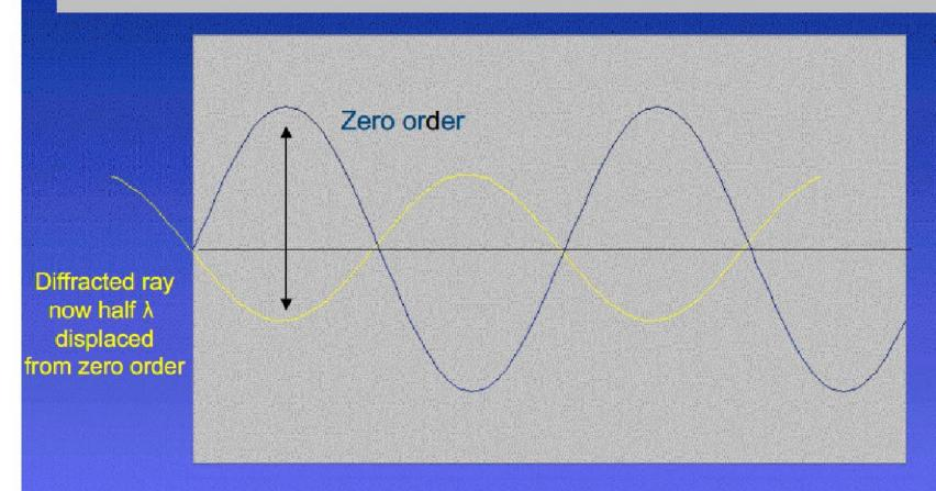
The diffracted ray is now in a position to interfere destructively with the zero order, but it is of lower amplitude
