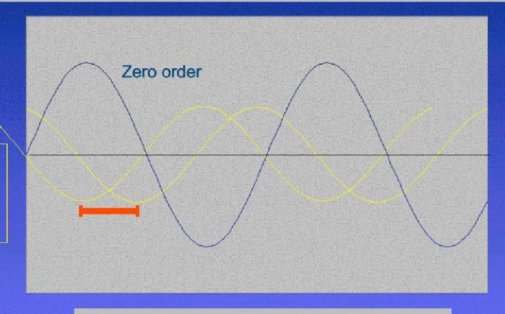
Diffracted ray shifted to left by a further  $\lambda/4$  by phase plate
