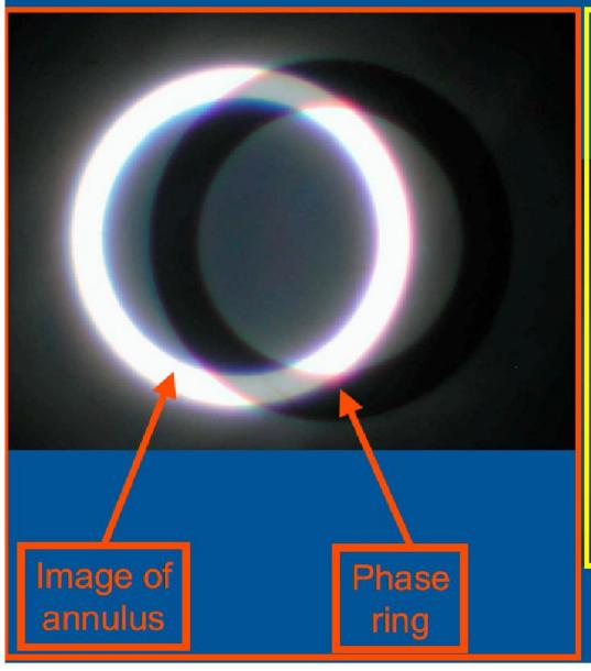
Illuminating annulus adjusted so that its image coincides with phase ring
