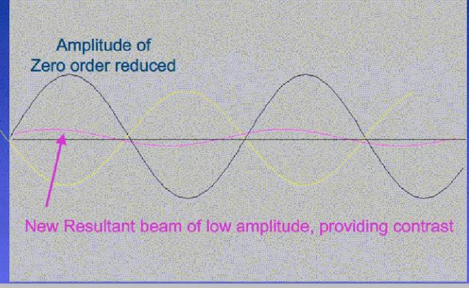
The diffraction pattern of our non-absorbing object has been converted into a diffraction pattern similar to that of an absorbing object - so the image looks like an image of an absorbing object.
